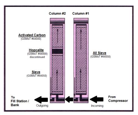
**Inspection:** Nothing lasts forever, not even stainless steel. Corrosive holes can develop in the canister after years of use or from improper maintenance. Therefore, periodic inspections of the wall of the tube should be conducted. This is best done in subdued light by holding a tank VIP light inside the canister. If any light is noted coming through the walls, the canister must be repaired or retired.
